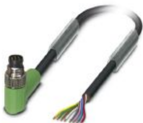
Sensor/actuator cable, 8-position, PUR halogen-free, black-gray RAL 7021, Plug angled M8, on free cable end, cable length: 10 m
