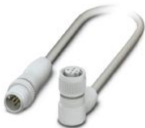
Sensor/actuator cable, 5-position, PP-EPDM halogen-free, gray RAL 7035, Plug straight M12, coding: A, on Socket angled M12, coding: A, with 3 LEDs, cable length: 0.6 m, Hygienic design, with plastic knurl
