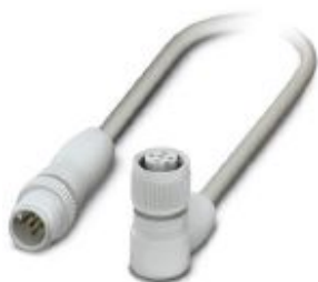
Sensor/actuator cable, 5-position, PP-EPDM halogen-free, gray RAL 7035, Plug straight M12, coding: A, on Socket angled M12, coding: A, cable length: 3 m, Hygienic design, with plastic knurl
