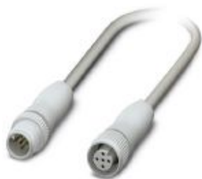
Sensor/actuator cable, 5-position, PP-EPDM halogen-free, gray RAL 7035, Plug straight M12, coding: A, on Socket straight M12, coding: A, cable length: 3 m, Hygienic design, with plastic knurl
