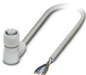
Sensor/actuator cable, 5-position, PP-EPDM halogen-free, gray RAL 7035, free cable end, on Socket angled M12, coding: A, cable length: 1.5 m, Hygienic design, with plastic knurl
