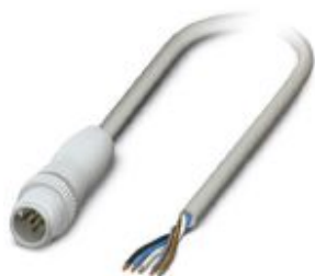
Sensor/actuator cable, 5-position, PP-EPDM halogen-free, gray RAL 7035, Plug straight M12, coding: A, on free cable end, cable length: 10 m, Hygienic design, with plastic knurl
