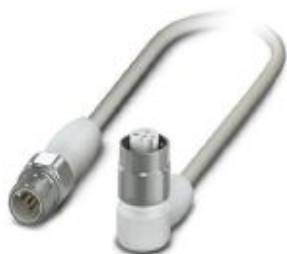
Sensor/actuator cable, 5-position, PP-EPDM halogen-free, gray RAL 7035, Plug straight M12, coding: A, on Socket angled M12, coding: A, cable length: 3 m, Hygienic design, with high-grade steel knurl
