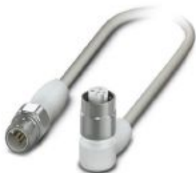
Sensor/actuator cable, 5-position, PP-EPDM halogen-free, gray RAL 7035, Plug straight M12, coding: A, on Socket angled M12, coding: A, cable length: 0.3 m, Hygienic design, with high-grade steel knurl
