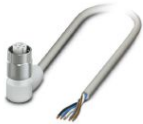
Sensor/actuator cable, 5-position, PP-EPDM halogen-free, gray RAL 7035, free cable end, on Socket angled M12, coding: A, with 3 LEDs, cable length: 1.5 m, Hygienic design, with high-grade steel knurl
