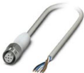
Sensor/actuator cable, 5-position, PP-EPDM halogen-free, gray RAL 7035, free cable end, on Socket straight M12, coding: A, cable length: 10 m, Hygienic design, with high-grade steel knurl
