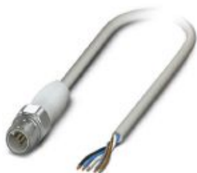
Sensor/actuator cable, 5-position, PP-EPDM halogen-free, gray RAL 7035, Plug straight M12, coding: A, on free cable end, cable length: 3 m, Hygienic design, with high-grade steel knurl
