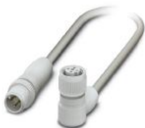
Sensor/actuator cable, 4-position, PP-EPDM halogen-free, gray RAL 7035, Plug straight M12, coding: A, on Socket angled M12, coding: A, with 3 LEDs, cable length: 1.5 m, Hygienic design, with plastic knurl
