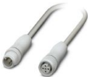
Sensor/actuator cable, 4-position, PP-EPDM halogen-free, gray RAL 7035, Plug straight M12, coding: A, on Socket straight M12, coding: A, cable length: 0.3 m, Hygienic design, with plastic knurl
