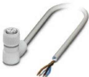
Sensor/actuator cable, 4-position, PP-EPDM halogen-free, gray RAL 7035, free cable end, on Socket angled M12, coding: A, cable length: 5 m, Hygienic design, with plastic knurl
