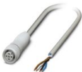
Sensor/actuator cable, 4-position, PP-EPDM halogen-free, gray RAL 7035, free cable end, on Socket straight M12, coding: A, cable length: 10 m, Hygienic design, with plastic knurl
