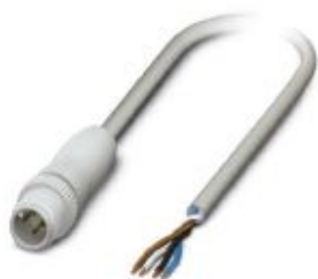
Sensor/actuator cable, 4-position, PP-EPDM halogen-free, gray RAL 7035, Plug straight M12, coding: A, on free cable end, cable length: 1.5 m, Hygienic design, with plastic knurl
