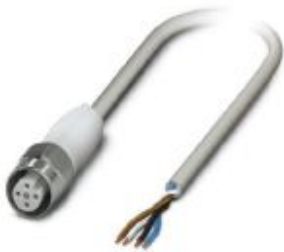
Sensor/actuator cable, 4-position, PP-EPDM halogen-free, gray RAL 7035, free cable end, on Socket straight M12, coding: A, cable length: 5 m, Hygienic design, with high-grade steel knurl
