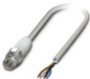
Sensor/actuator cable, 4-position, PP-EPDM halogen-free, gray RAL 7035, Plug straight M12, coding: A, on free cable end, cable length: 3 m, Hygienic design, with high-grade steel knurl
