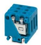
Mini feed-through terminal block, nom. voltage: 500 V, nominal current: 17.5 A, connection method: Screw connection, number of connections: 2, cross section: 0.2 mm² - 2.5 mm², AWG: 24 - 14, width: 5 mm, color: blue, mounting type: NS 15
