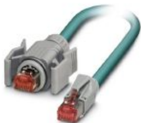
Assembled Ethernet cable, CAT6, shielded, 4-pair, AWG 26 stranded (7-wire), RAL 5021 (water blue), RJ45 connector/IP67, gray on RJ45 connector/IP20, line, length 6.5 m
