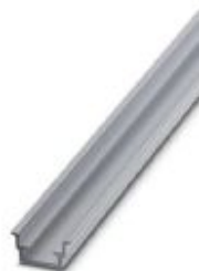
DIN rail, unperforated, Standard profile, width: 35 mm, height: 15 mm, similar to EN 60715, material: Aluminum, uncoated, length: 1000 mm, color: silver
