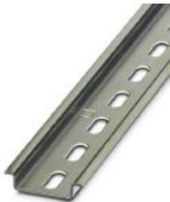
DIN rail perforated, Standard profile, width: 35 mm, height: 7.5 mm, acc. to EN 60715, material: Steel, galvanized, passivated with a thick layer, length: 755 mm, color: silver
