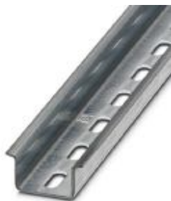
DIN rail perforated, Standard profile, width: 35 mm, height: 15 mm, similar to EN 60715, material: Steel, galvanized, length: 2000 mm, color: silver
