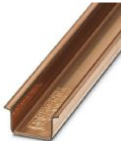
DIN rail, unperforated, Standard profile, width: 35 mm, height: 15 mm, similar to EN 60715, material: Copper, uncoated, length: 2000 mm, color: copper-colored
