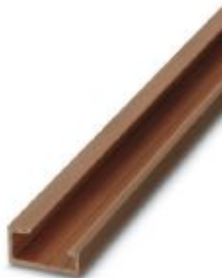
DIN rail, unperforated, G profile, width: 32 mm, height: 15 mm, similar to EN 60715, material: Copper, uncoated, length: 2000 mm, color: copper-colored
