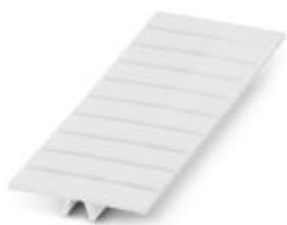
Unprinted zack marker strip, special surface specifications for labeling with UV systems, 10-section, lettering field size: 8 x 27 mm, color: white
