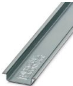
DIN rail, unperforated, Standard profile, width: 35 mm, height: 7.5 mm, acc. to EN 60715, material: Aluminum, uncoated, length: 2000 mm, color: silver
