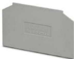
Partition plate, length: 69 mm, width: 1.5 mm, height: 40.8 mm, color: gray
