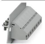
Panel feed-through terminal block, connection method: Screw connection with tension sleeve, Cable lug connection, number of positions: 1, load current: 150 A, cross section: 16 mm² - 50 mm², connection direction of the conductor to plug-in direction: -90 °, width: 18.8 mm, color: gray
