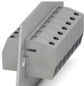
Panel feed-through terminal block, connection method: Screw connection with tension sleeve, Screw connection with tension sleeve, number of positions: 1, load current: 101 A, cross section: 6 mm<sup>2</sup> - 35 mm<sup>2</sup>, connection direction of the conductor to plug-in direction: 0 °, width: 15.1 mm, color: green-yellow
