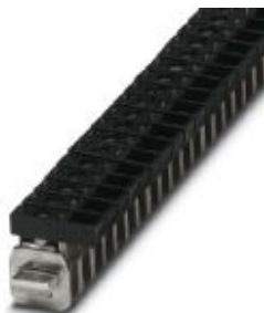
Connection terminal block, connection method: Screw connection, load current: 41 A, cross section: 0.5 mm 2 - 6 mm 2 , width: 7 mm, color: black
