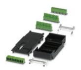
Bus connector set consisting of  $2 \times 10$ -pos. connectors, plastic upper part and base, plus metal clamp for mounting on DIN rail, without PCB
