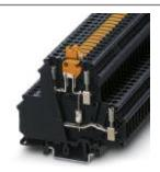
Double-level modular terminal block with suppressor diode as surge protection between both levels, disconnect knife in the upper level, nominal voltage: 60 V AC, for mounting on NS 32 or NS 35/7.5, closed housing, terminal width: 6.2 mm, terminal height: 68 mm
