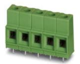
PCB terminal block, nominal current: 76 A, nom. voltage: 1000 V, pitch: 10.16 mm, number of positions: 2, connection method: Screw connection with tension sleeve, mounting: Wave soldering, conductor/PCB connection direction: 0 °, color: green
