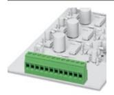
PCB terminal block, nominal current: 24 A, nom. voltage: 400 V, pitch: 5.08 mm, number of positions: 6, connection method: Screw connection with tension sleeve, mounting: Wave soldering, conductor/PCB connection direction: 0 $^{\circ}$ , color: green
