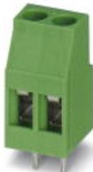
PCB terminal block, nominal current: 24 A, nom. voltage: 400 V, pitch: 5.08 mm, number of positions: 3, connection method: Screw connection with tension sleeve, mounting: Wave soldering, conductor/PCB connection direction: 0 °, color: green
