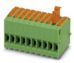
PCB terminal block, nominal current: 15 A, nom. voltage: 320 V, pitch: 5.08 mm, number of positions: 1, connection method: Screw connection with tension sleeve, mounting: Wave soldering, conductor/PCB connection direction: 0 °, color: green
