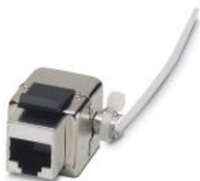
RJ45 socket insert, modular (Keystone), CAT5e, 8-pos., shielded, with cable connection (LSA), for solid wires AWG 26 ... 22
