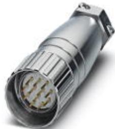
Cable connector, with Pg11 connection thread, straight, shielded: yes, Screw locking, M23, No. of pos.: 8+1, type of contact: Pin, Crimp connection, cable diameter range: 6.5 mm ... 7.5 mm
