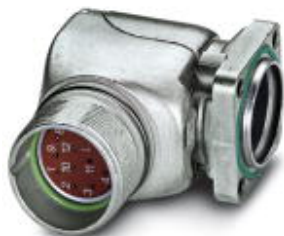
Device connector, front mounting, angled rotatable, Screw locking, M23, number of positions: 17, type of contact: Pin, Crimp connection, Axial O-ring, 4x Ø 3.2, shielded: yes, flange dimensions: 26 mm x 26 mm
