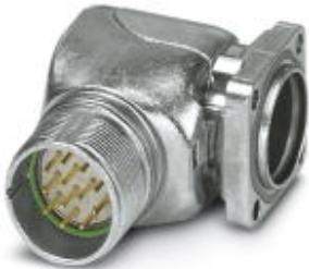
Device connector for front wall, angled rotatable, shielded: yes, Screw locking, M23, Axial O-ring, 4x Ø 3.2
