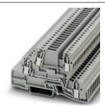
Installation level terminal block, Screw connection, cross section: 0.2 mm² - 4 mm², AWG: 24 - 12, width: 6.2 mm, color: gray, mounting type: NS 35/7,5, NS 35/15
