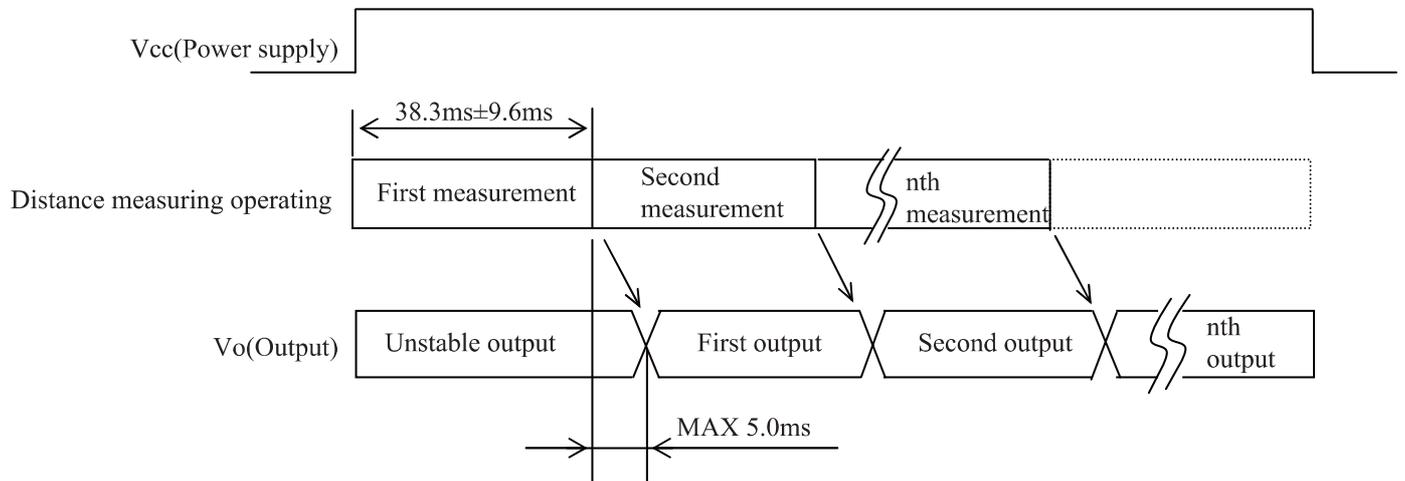
**Fig. 2 Example of distance measuring characteristics(output)**
