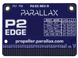
The P2 Edge Module is a simple way to get started with the Propeller 2 multicore microcontroller. In addition to speeding development, this module provides an optimal P2 building block for system integrators and designers to include in their products.
