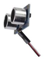
The bending of the connector assembly provides the necessary space for the two sensors to be mounted in close proximity to each other.
