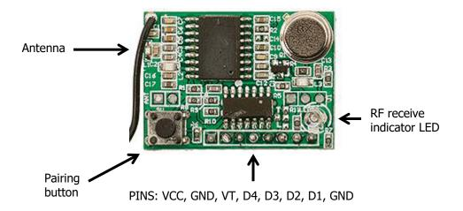
The Receiver Board has a pre-soldered antenna in "ANT2". To add even more range to the receiver you can add your own antenna to "ANT1" on the receiver board.
