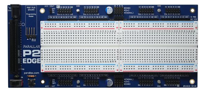
The Propeller 2 Edge Module Breadboard provides a convenient rapid prototyping solution for experimenting and developing with the Propeller 2 microcontroller.
