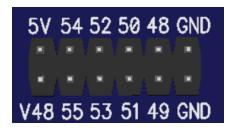
There are two special usage edge header banks which do not supply the 5V output. Refer to the details here: I/O Pin Breakout Edge Headers (without 5V output)
