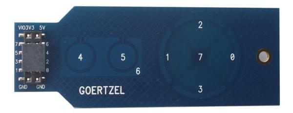
The Goertzel experimenter board features (Rev B) pads for non-contact switching or position sensing. Pads 4, 5 and 6 are typically used as on/off (switch style) inputs, whereas 0,1,2,3 and 7 for a set of Goertzel input pads.
