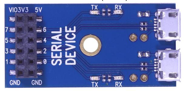
The Serial Device accessory board has two microUSB-type sockets, each with two activity LEDs.
