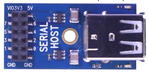
The Serial Host accessory board has twin USB-type A sockets, each protected with a current-limited load switch that allows up to 500 mA continuous current, subject to overall available system power. Additional protection includes reverse current blocking, short-circuit protection, over temperature protection and VBUS soft start.
