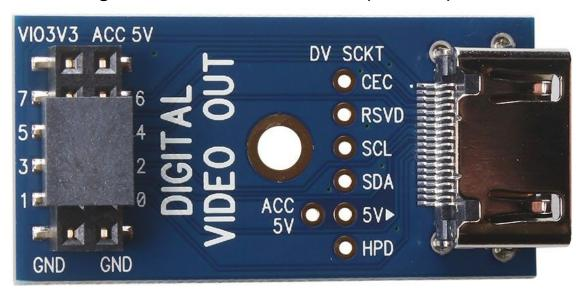
The Digital Video Out Accessory Board provides an HDMI-type connector which can be used for experimenting with various video standards. The signal pins which are connected to the P2-EVAL header are shown in this table:
