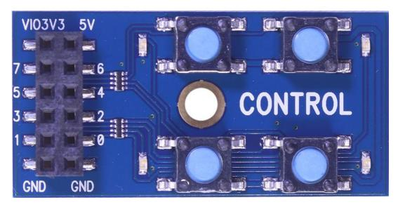
The Control accessory board includes four push-buttons and four blue LEDs.
