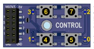
The push-buttons allow simple digital input control of other circuits or processes. Each active-high push-button has a 470  $\Omega$  series resistor to allow the I/O pin to be driven low while the button is asserted.
