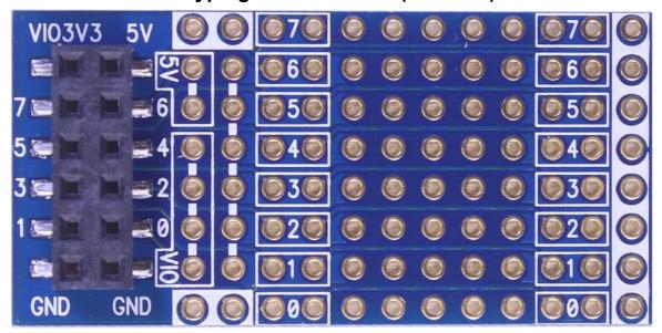
The Mini Prototyping Add-on Board provides an 8x12 grid of plated thru-holes.
