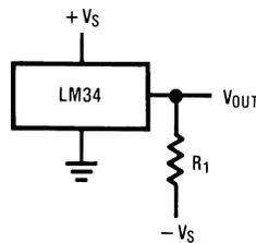
$$\begin{aligned} \text{CHOOSE } R_1 &= (-V_S)/50 \mu\text{A} \\ V_{OUT} &= +3,000 \text{ mV AT } +300^\circ\text{F} \\ &= +750 \text{ mV AT } +75^\circ\text{F} \\ &= -500 \text{ mV AT } -50^\circ\text{F} \end{aligned}$$
