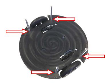
**Step 2**: Place the Top Deck onto the standoffs, making sure that the counter-sunk holes are face-up. Secure the deck with the four included ¼"- 20 x 5/8" flat-head screws.
